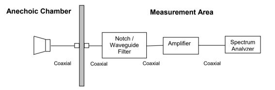
Measurement set up for Radiated Emission Test
