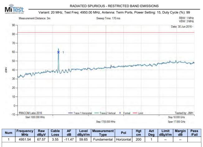
Test Notes: EUT A5c SN: 2118161852 on 150cm table, powered by Mimosa POE PS 502-00002. Ports Term with 50 ohms
