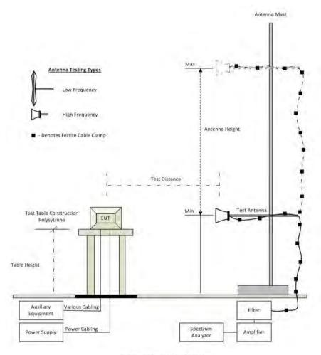
Radiated Emission Test Setup
