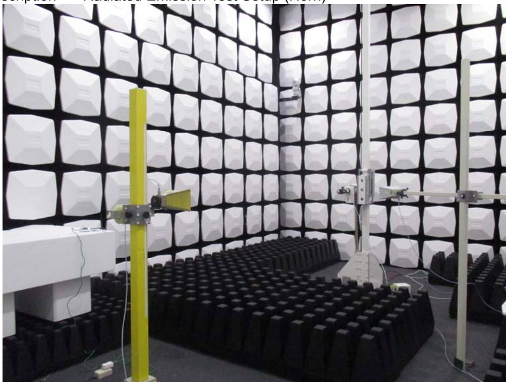
Description : Radiated Emission Test Setup (Horn)
