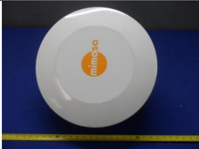
25dBi Antenna – Top View
