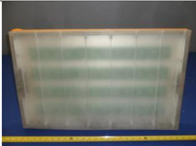
0dBi Antenna – Top View
