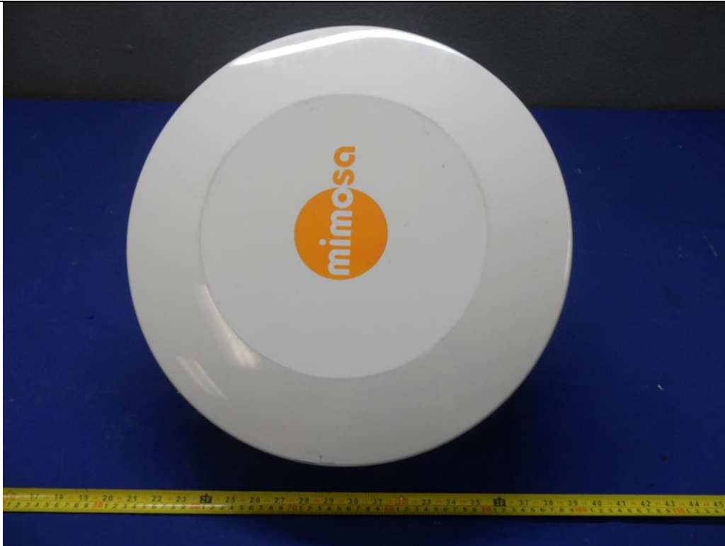
25dBi Antenna – Top View
