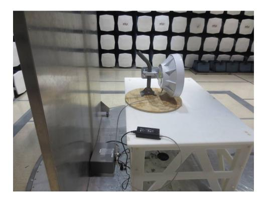
14.10 AC Line Conducted Emissions - Front View -0 dBi Antenna
