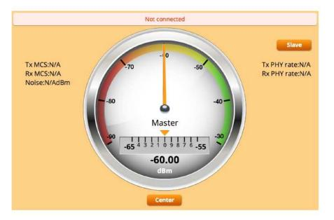
Current **Tx MCS (Modulation and Coding Scheme)** and **Rx MCS** rate (if associated) corresponding **Tx PHY (Physical Layer** Interface) rate and **Rx PHY rate** are shown.
