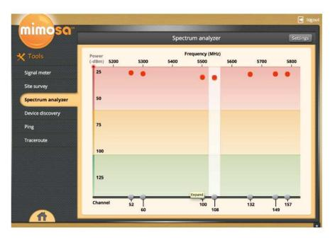
Unlike many wireless spectrum analyzers, the Mimosa device continually captures interfering signal levels across the spectrum without impacting ongoing link traffic.
