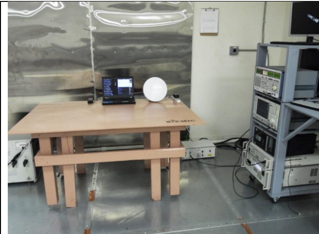
AC Line Conducted Emissions – Front View
