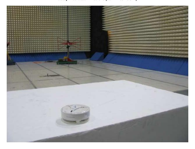
Setup: Radiated Emissions (1Ghz to 18Ghz)
