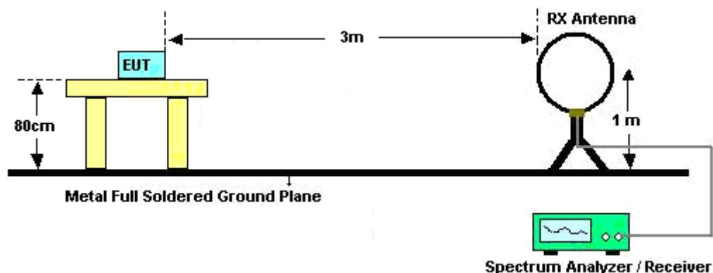
For radiated emissions from 30MHz to 1GHz
