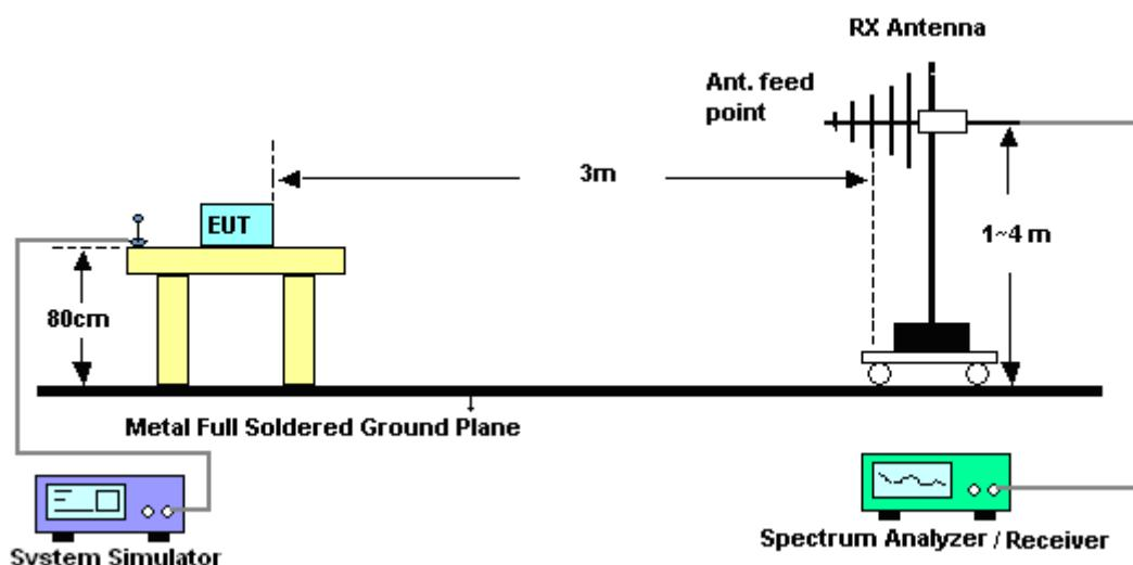
For radiated emissions from 1GHz to 18GHz
