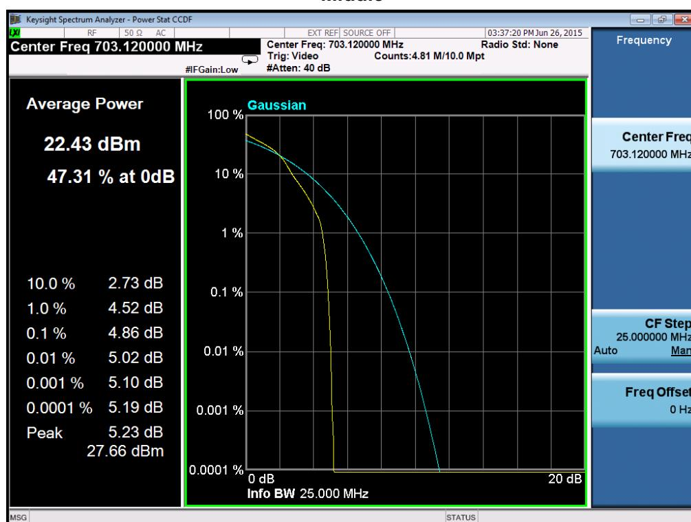
**Peak to Average Ratio of Configuration-16-QAM-10M/1RB channel
