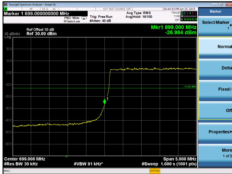
**Band Edge on Configuration QPSK-3M / 15RB Channel**
