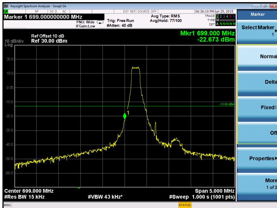
**Band Edge on Configuration QPSK-1.4M / 1RB Channel**
