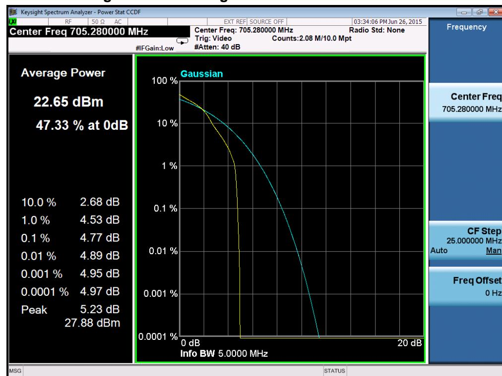
**Peak to Average Ratio of Configuration-16-QAM-5M/1RB channel
