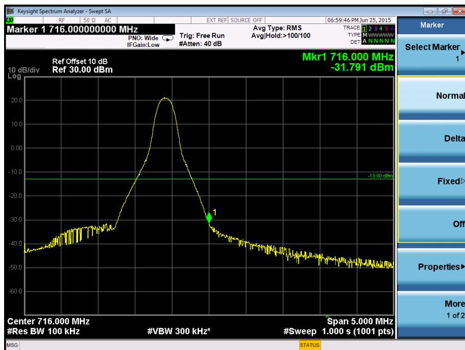
**Band Edge on Configuration QPSK-10M / 50RB Channel
