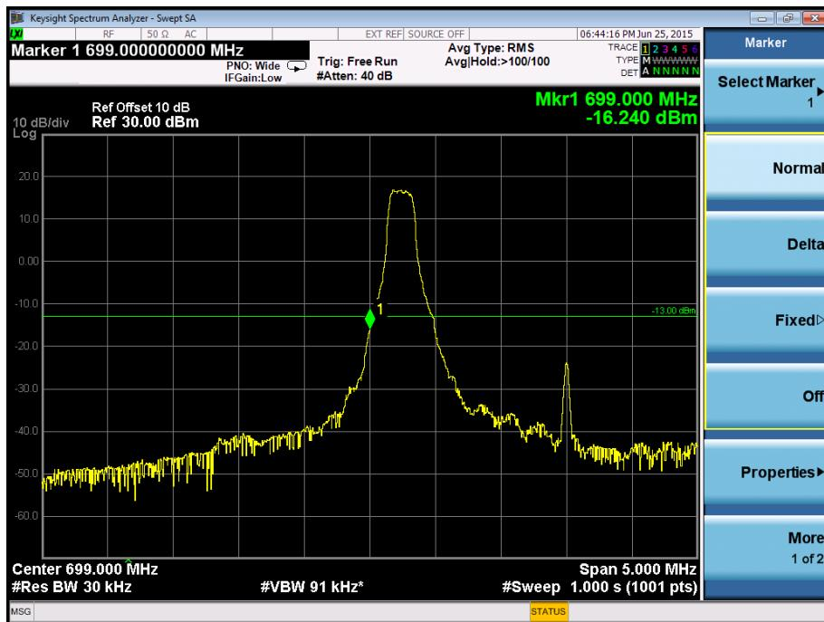
**Band Edge on Configuration QPSK-3M / 1RB Channel
