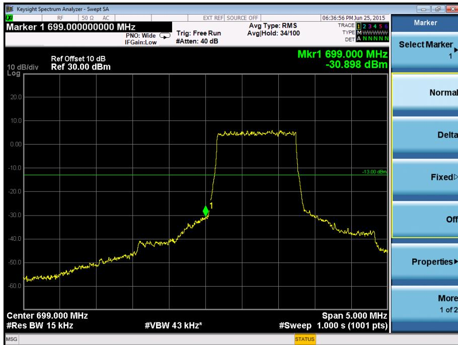
**Band Edge on Configuration QPSK-1.4M / 6RB Channel
