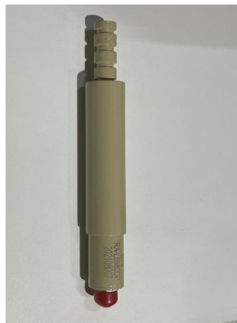
Fig 4 dipole model RA-L6989DP frequency 6900~8000 MHz
