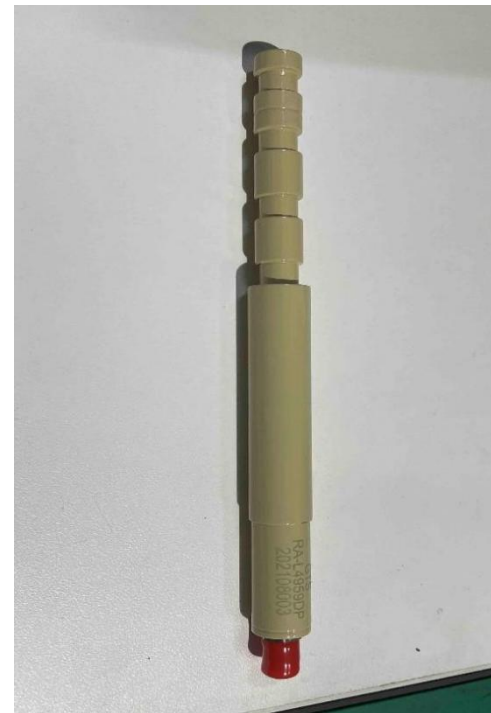
Fig 2 dipole model RA-L4959DP frequency 4900~5900 MHz
