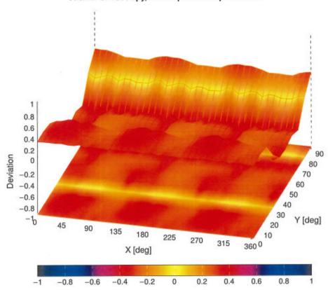
Probe isotropy for E<sub>tot</sub>: probe rotated  $\phi = 0^\circ$  to 360°, tilted from field propagation direction  $\vec{k}$  Parallel to the field propagation ( $\psi = 0^\circ - 90^\circ$ ) at 30 GHz: deviation within  $\pm 0.37$  dB Parallel to the field propagation ( $\psi = 0^\circ - 90^\circ$ ) at 60 GHz: deviation within  $\pm 0.39$  dB
