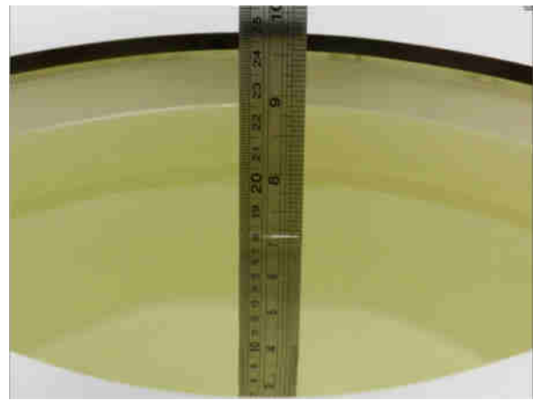
Fig 10.2 Photo of Liquid Height for Body SAR
