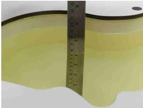
Fig 10.1 Photo of Liquid Height for Head SAR
