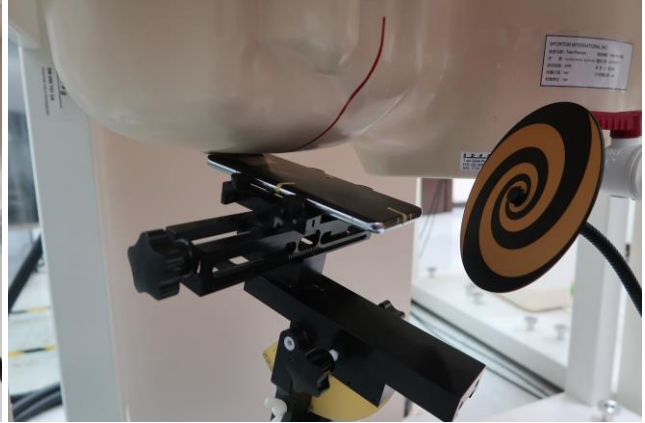
Head, Right Tilted, Separation distance 0mm
