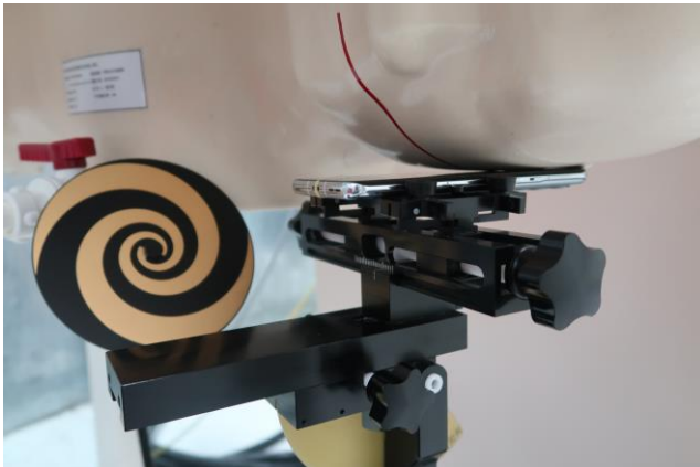
Head, Left Check, Separation distance 0mm
