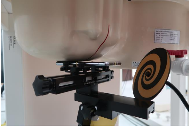
Head, Right Check, Separation distance 0mm
