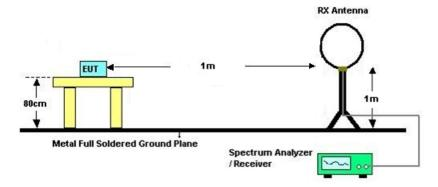
Note: There is a comparison data of both open-field test site and alternative test site - semi-Anechoic chamber according to 414788 D01 Radiated Test Site v01r01, and the result came out very similar.
