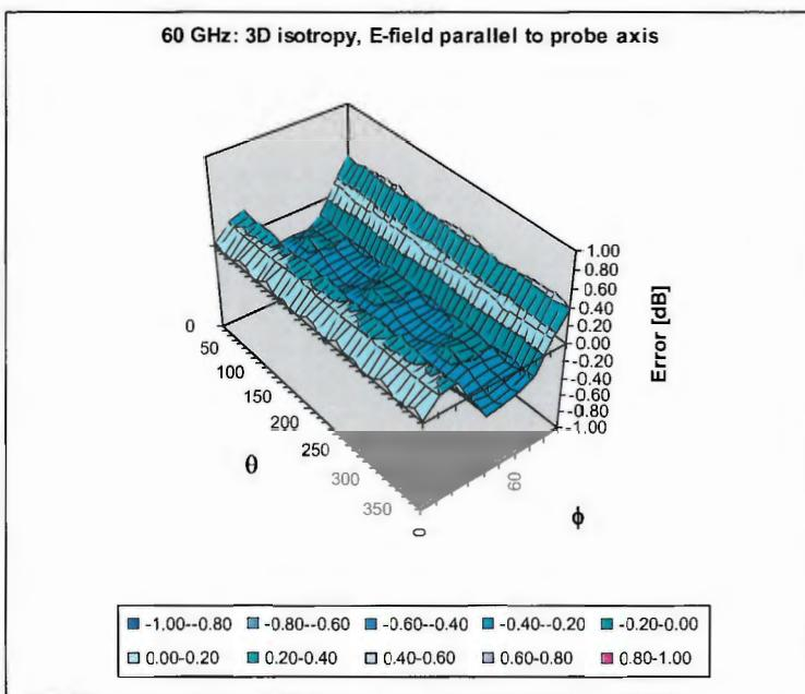
Probe isotropy for  $E_{\text{tot}}$ : probe rotated  $\varphi = 0^\circ$  to  $360^\circ$ , tilted from field propagation direction  $\vec{k}$
