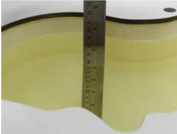
Fig 10.1 Photo of Liquid Height for Head SAR
