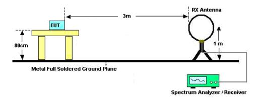
For radiated emissions from 30MHz to 1GHz
