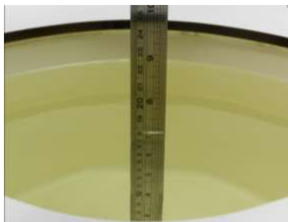
Fig 10.2 Photo of Liquid Height for Body SAR
