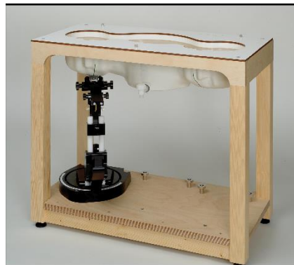
Picture C.10: SAM Twin Phantom
