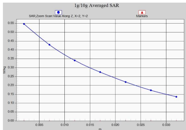
Z-Scan at power reference point (850 MHz)
