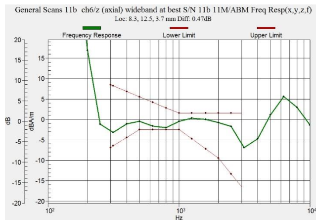
Figure C.24 Frequency Response of WiFi-2.4G - OTT VoIP
