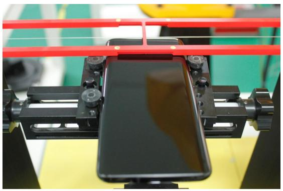
Picture 2: EUT Positioning for RF/T-coil
