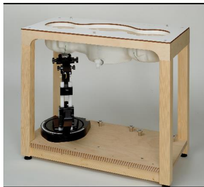
Picture C.10: SAM Twin Phantom
