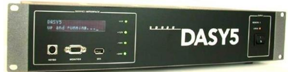
Picture C.8 Server for DASY 5
