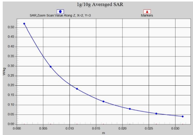
Z-Scan at power reference point (LTEB7)
