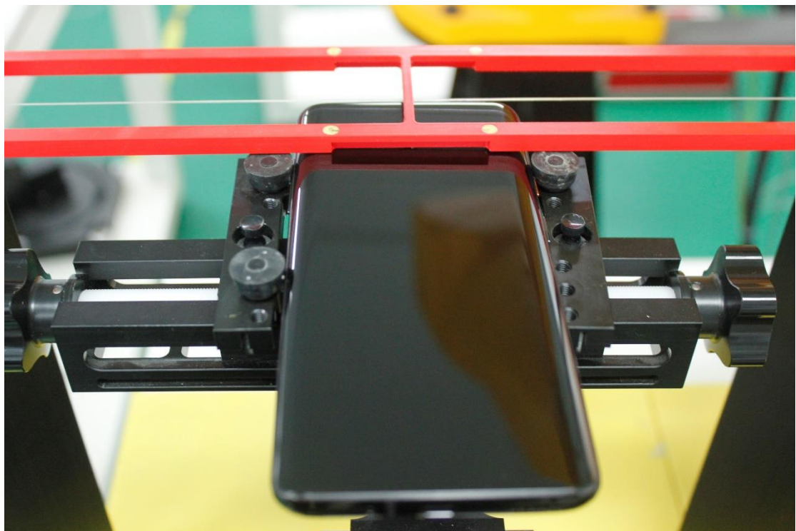
Picture 2: EUT Positioning for RF/T-coil
