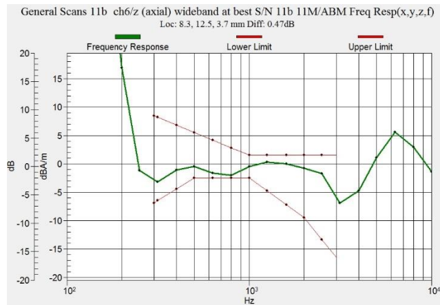
Figure C.26 Frequency Response of WiFi-2.4G - OTT VoIP
