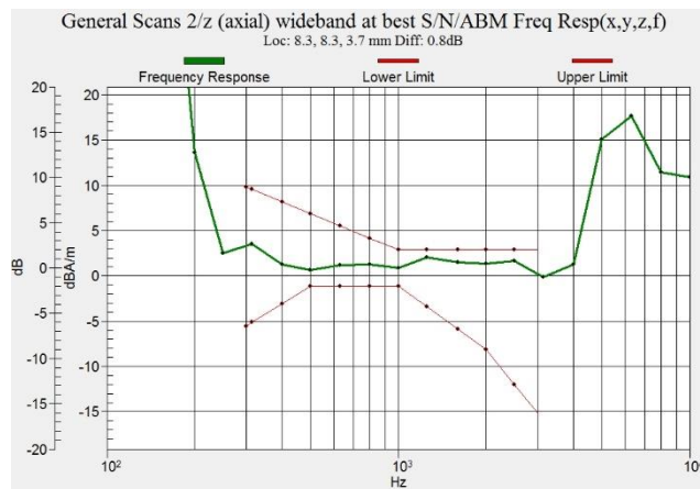
Figure C.8 Frequency Response of CDMA BC10
