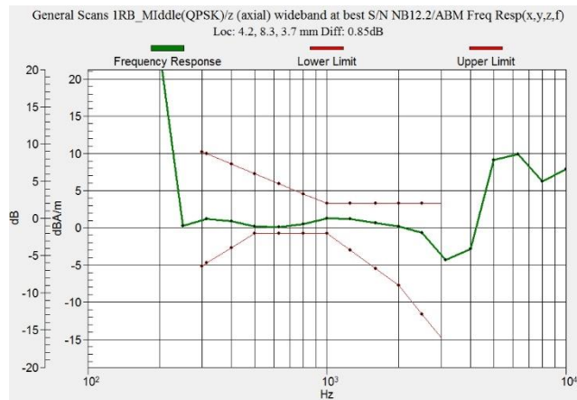
Figure C.17 Frequency Response of LTE B41 Power Class 2
