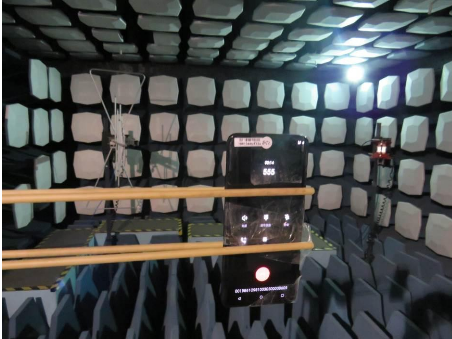
Pic.1 Radiated spurious emission
