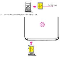
Please use the SIM Tray Ejector (found in the box) to remove the SIM tray from the device and insert **Nano SIM** cards in the tray.
