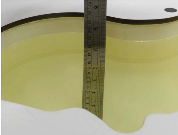
Fig 10.1 Photo of Liquid Height for Head SAR
