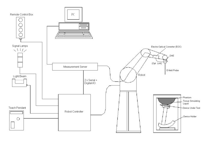
The DASY system for performing compliance tests consists of the following items:
