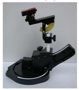
The positioning system allows obtaining cheek and tilting position with a very good accuracy. Incompliance with CENELEC, the tilt angle uncertainty is lower than 1°.
