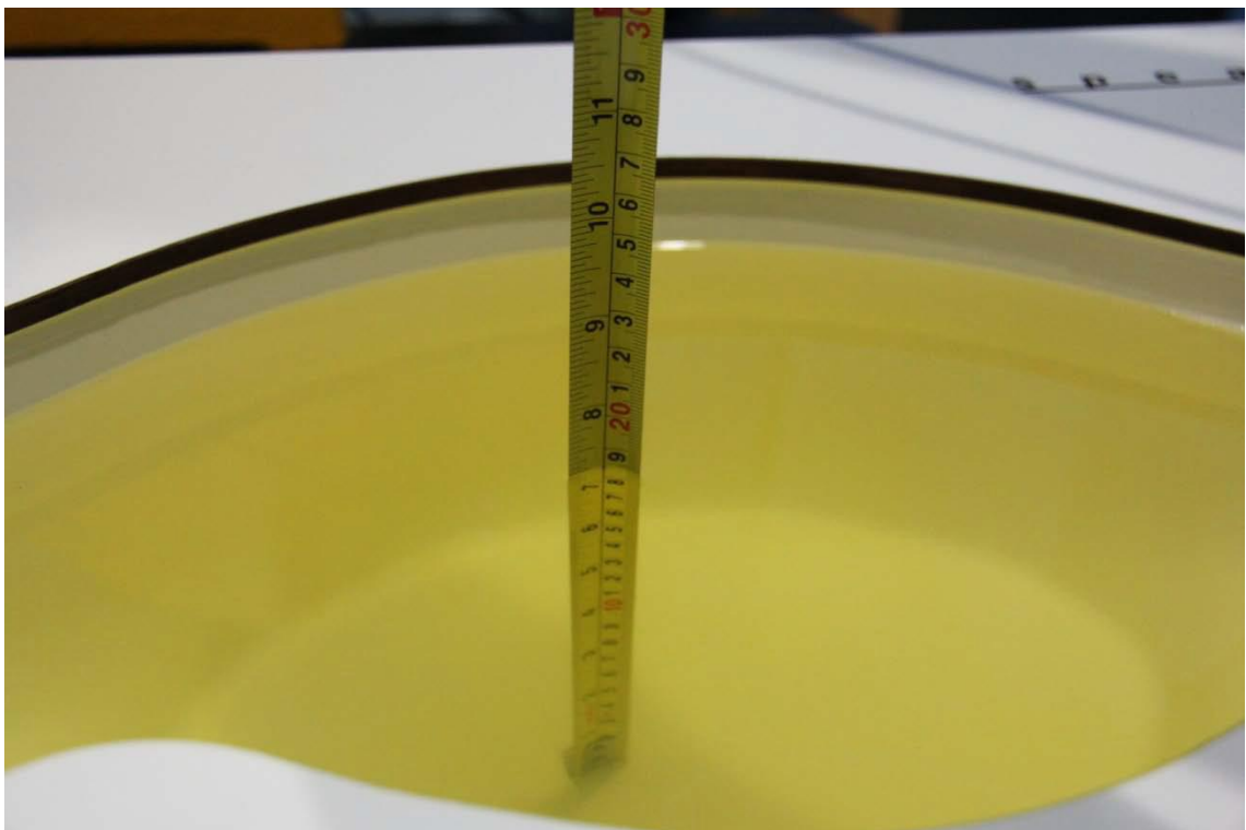
Picture 7-1: Liquid depth in the Flat Phantom(2450MHz)
