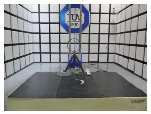
radiated spurious emission 9KHz-30MHz
