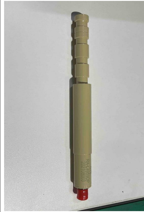
Fig 2 dipole model RA-L4959DP frequency 4900~5900 MHz
