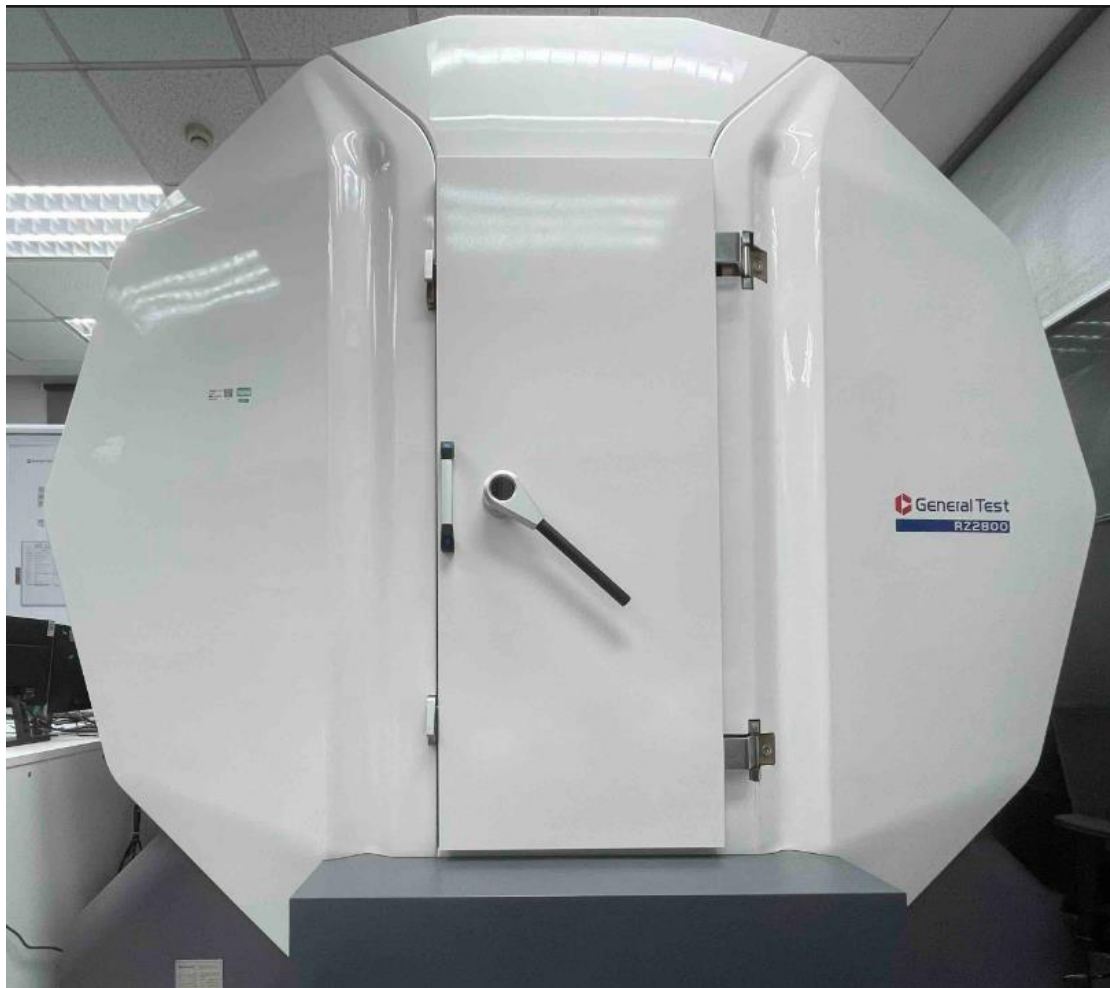
Fig. 5. The fully anechoic chamber
