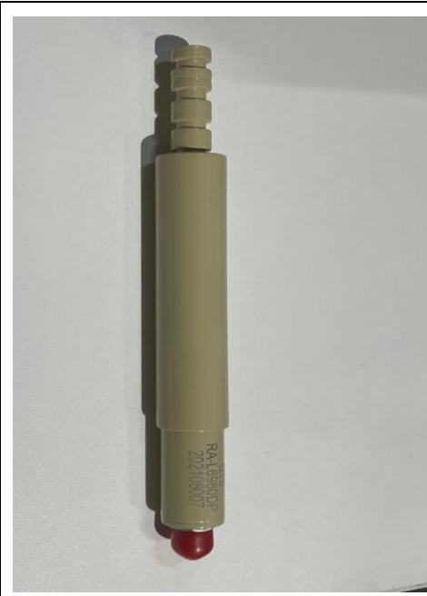
Fig 4 dipole model RA-L6989DP frequency 6900~8000 MHz
