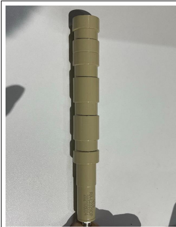
Fig 1 dipole model RA-L2329DP frequency 2300~2900 MHz
