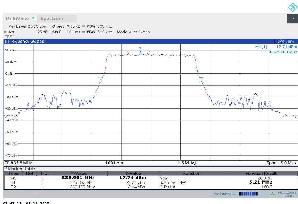
**n5,5MHz Bandwidth,DFT-s-QPSK (-26dBc BW)**
