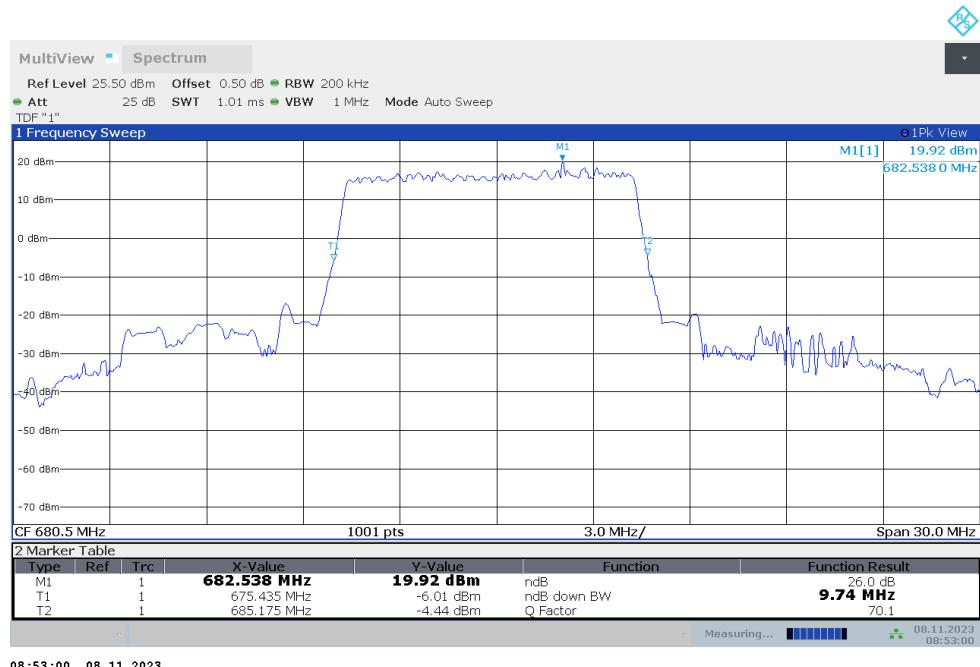
**n71,10MHz Bandwidth,DFT-s-QPSK (-26dBc BW)**
