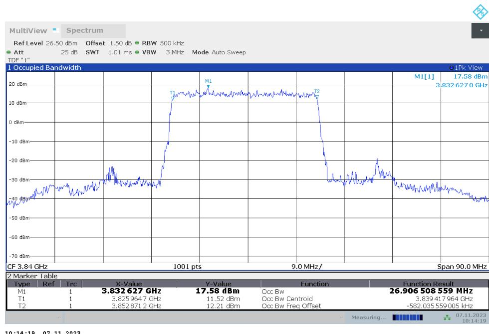
**n77H,30MHz Bandwidth,DFT-s-QPSK (99% BW)**
