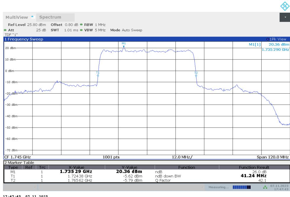
**n66,40MHz Bandwidth,DFT-s-QPSK (-26dBc BW)**
