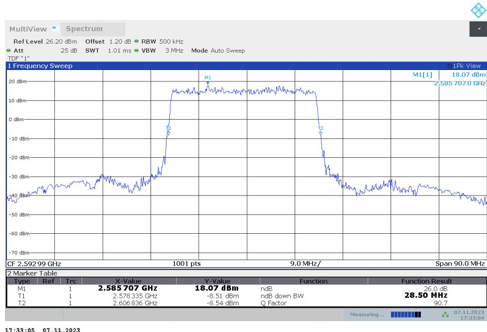
**n41,30MHz Bandwidth,DFT-s-QPSK (-26dBc BW)**
