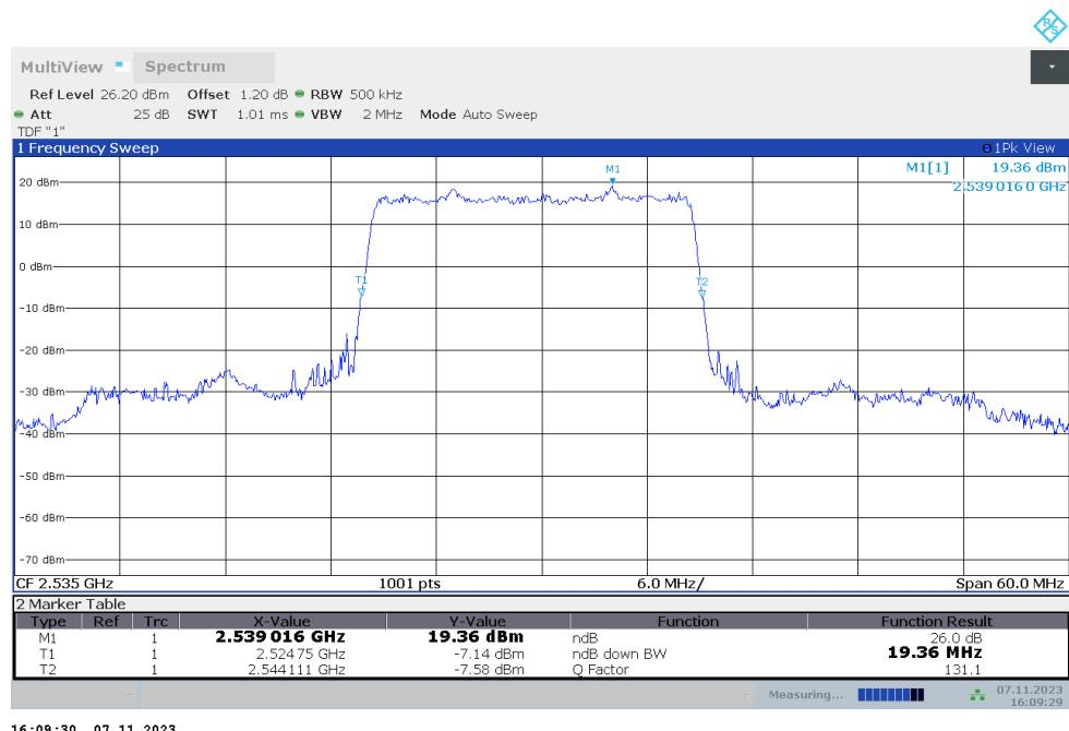
**n7,20MHz Bandwidth,DFT-s-QPSK (-26dBc BW)**
