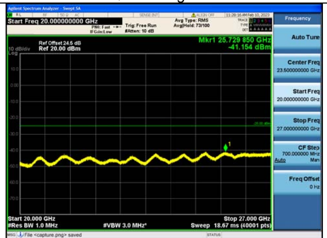
Band41C-20G-27G / 5MHz+20MHz / 25RB+100RB / QPSK / High CH
