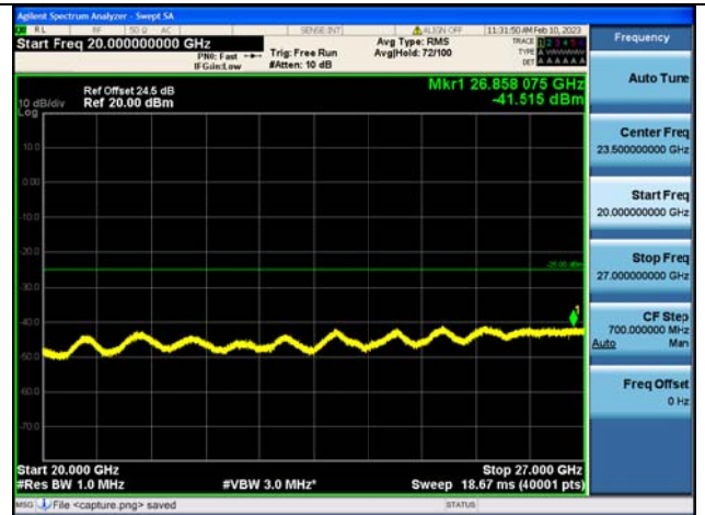
Band41C-20G-27G / 10MHz+15MHz /1RB+1RB/ QPSK / High CH
