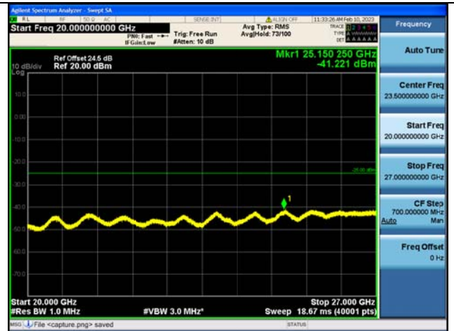
Band41C-20G-27G / 15MHz+10MHz /1RB+1RB/ QPSK / High CH
