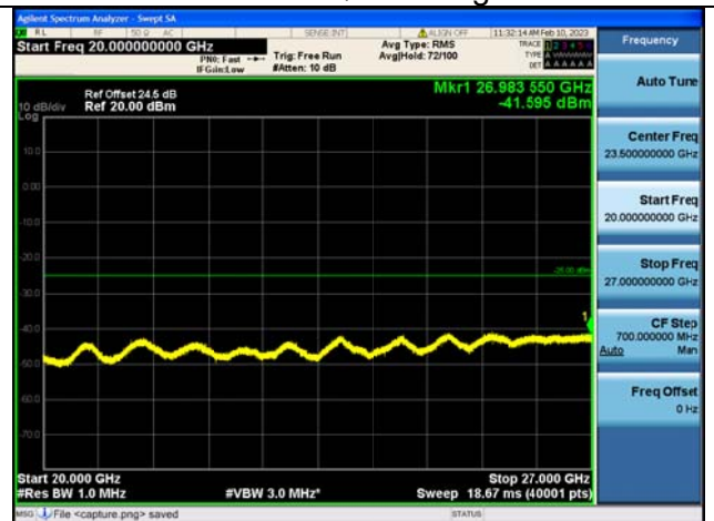
Band41C-20G-27G / 10MHz+15MHz /1RB+1RB/ QPSK / High CH
