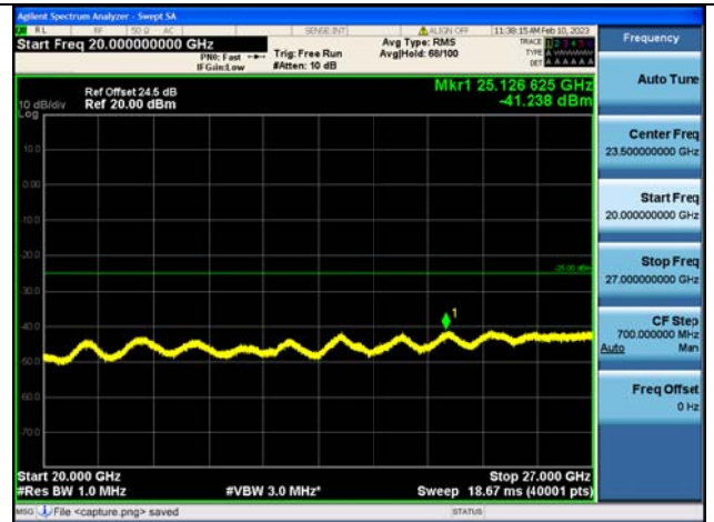
Band41C-20G-27G / 15MHz+15MHz /1RB+1RB/ QPSK / High CH
