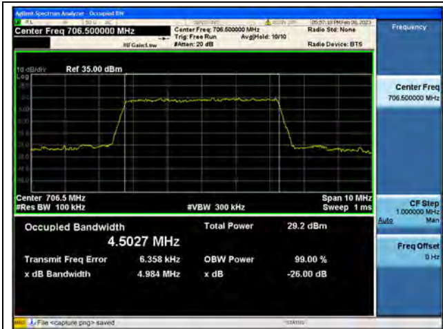
Band17 / 5MHz / QPSK/ Low CH
