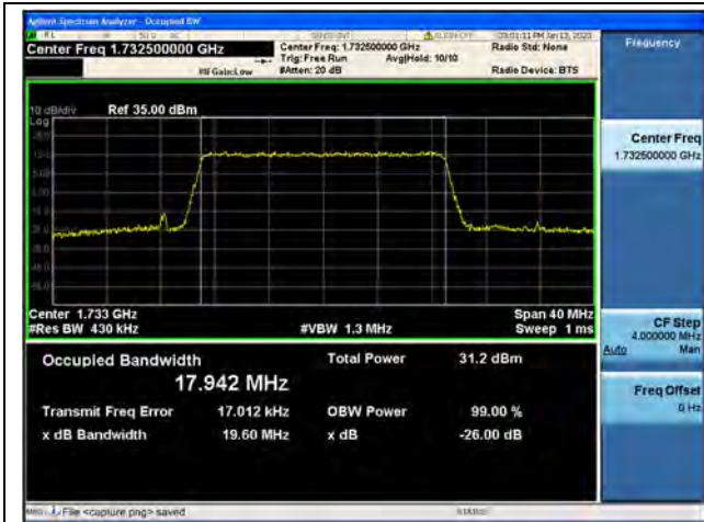
Band4 / 20MHz / QPSK/ Mid CH
