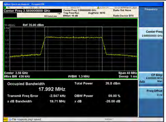
Band7 / 20MHz / 64QAM/ High CH
