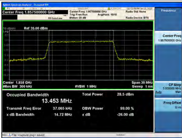
Band2 / 15MHz / 64QAM/ Low CH
