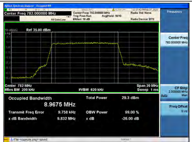
Band13 / 10MHz / 64QAM/ High CH
