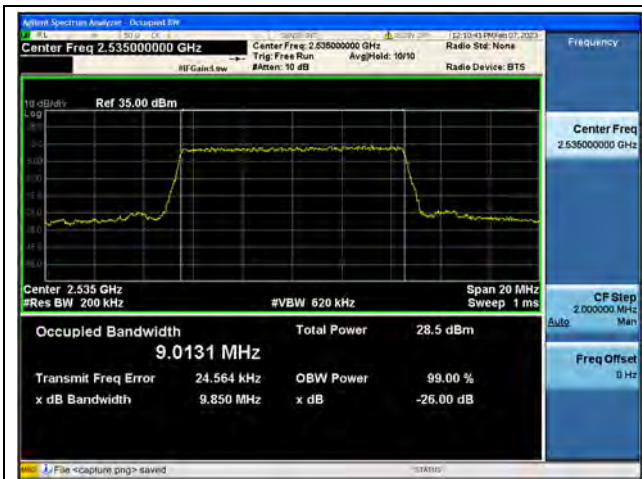
Band7 / 10MHz / QPSK/ Mid CH
