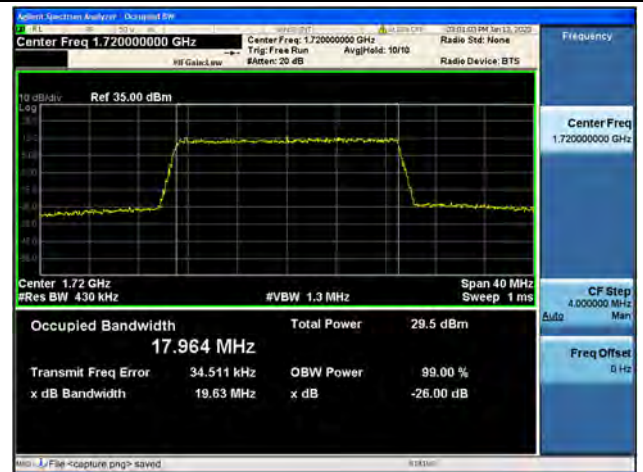
Band4 / 20MHz / 64QAM/ Low CH
