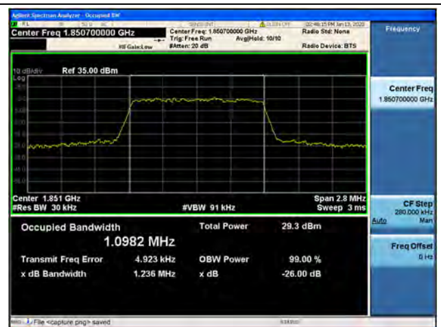
Band2 / 1.4MHz / 16QAM/ Low CH
