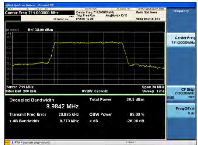
Band12 / 10MHz / QPSK/ High CH
