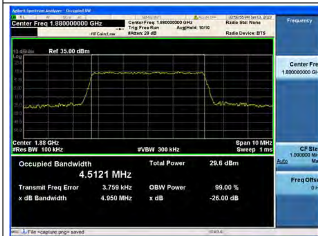
Band2 / 5MHz / 16QAM/ Mid CH
