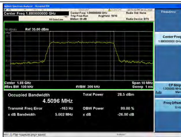
Band2 / 5MHz / 64QAM/ Mid CH
