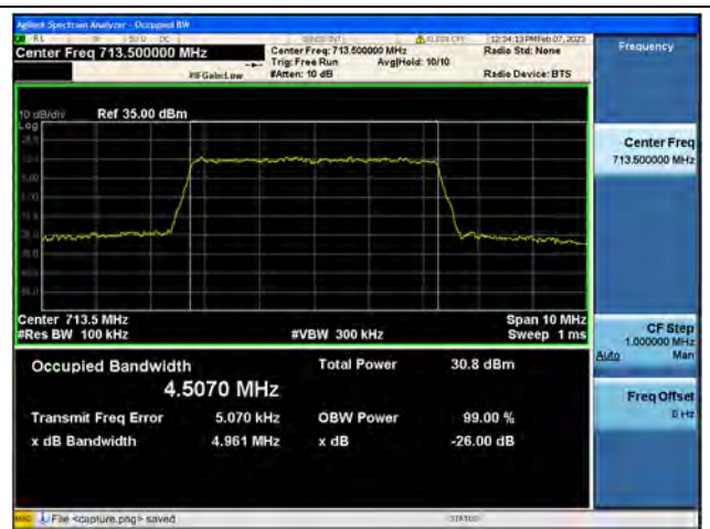
Band12 / 5MHz / 16QAM/ High CH
