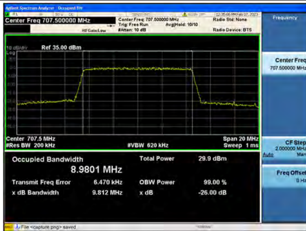
Band12 / 10MHz / 64QAM/ Mid CH
