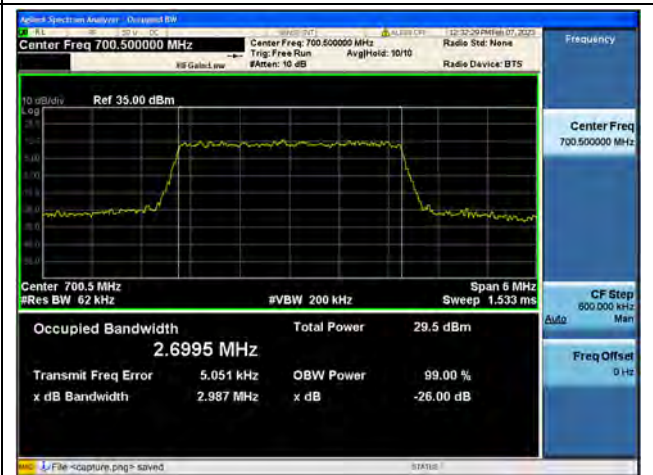
Band12 / 3MHz / 64QAM/ Low CH
