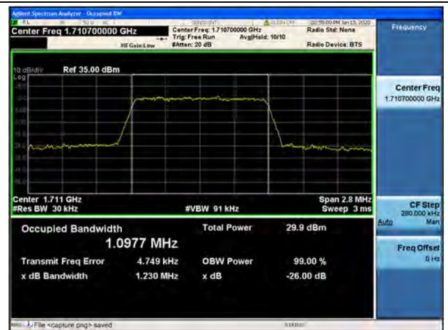
Band4 / 1.4MHz / 16QAM/ Low CH
