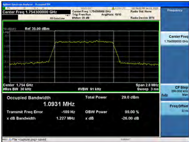
Band4 / 1.4MHz / 64QAM/ High CH
