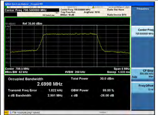
Band12 / 3MHz / QPSK/ Low CH
