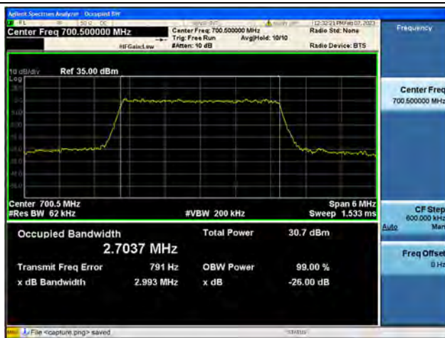
Band12 / 3MHz / 16QAM/ Low CH
