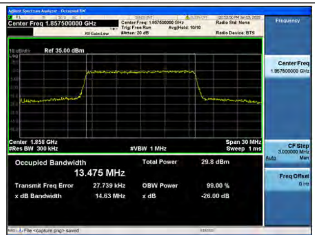
Band2 / 15MHz / 16QAM/ Low CH
