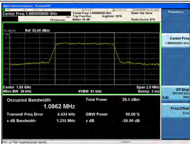
Band2 / 1.4MHz / 16QAM/ Mid CH
