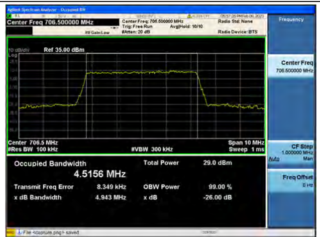
Band17 / 5MHz / 16QAM/ Low CH
