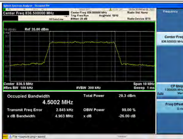
Band5 / 5MHz / 16QAM/ Mid CH
