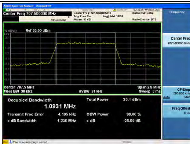
Band12 / 1.4MHz / 16QAM/ Mid CH
