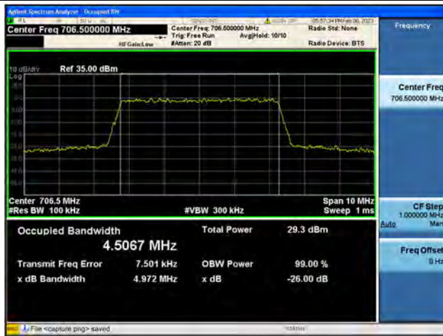
Band17 / 5MHz / 64QAM/ Low CH
