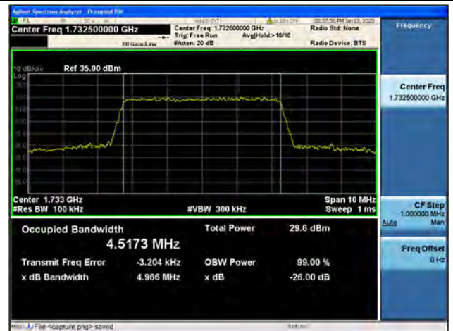
Band4 / 5MHz / 64QAM/ Mid CH
