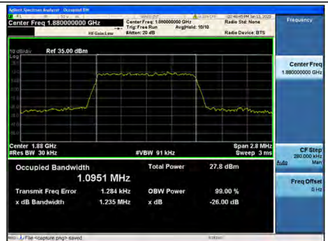
Band2 / 1.4MHz / 64QAM/ Mid CH
