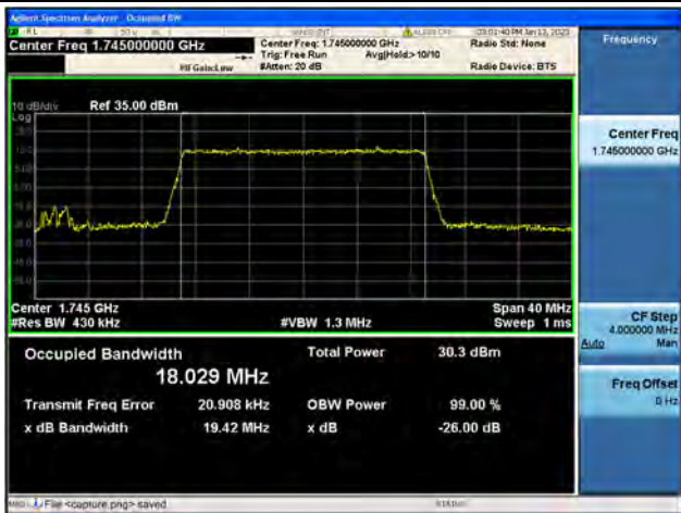
Band4 / 20MHz / 16QAM/ High CH
