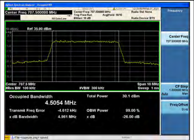
Band12 / 5MHz / 64QAM/ Mid CH
