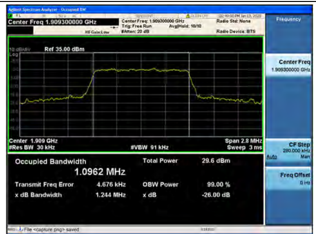
Band2 / 1.4MHz / 16QAM/ High CH
