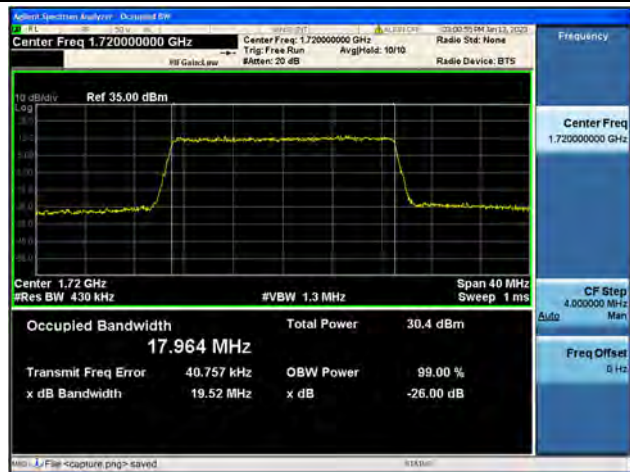
Band4 / 20MHz / 16QAM/ Low CH
