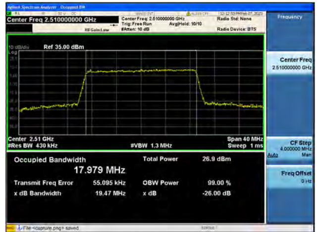
Band7 / 20MHz / 64QAM/ Low CH
