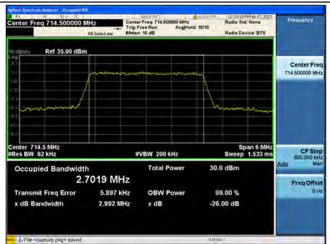
Band12 / 3MHz / 64QAM/ High CH
