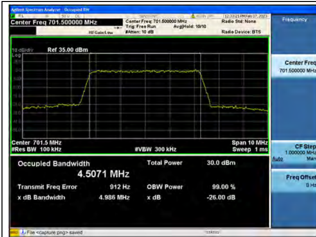
Band12 / 5MHz / QPSK/ Low CH
