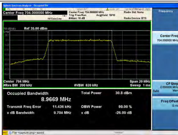
Band12 / 10MHz / 16QAM/ Low CH
