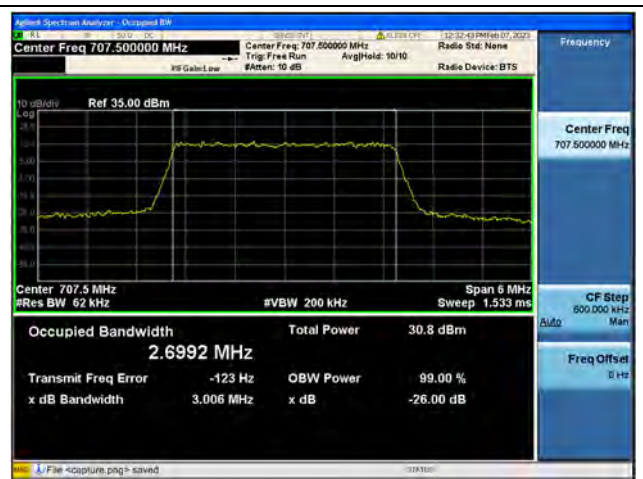
Band12 / 3MHz / 16QAM/ Mid CH
