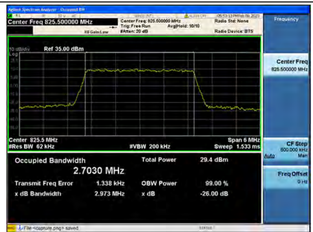
Band5 / 3MHz / 64QAM/ Low CH
