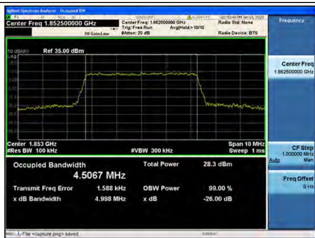
Band2 / 5MHz / 64QAM/ Low CH
