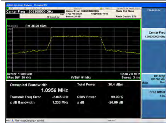
Band2 / 1.4MHz / QPSK/ High CH
