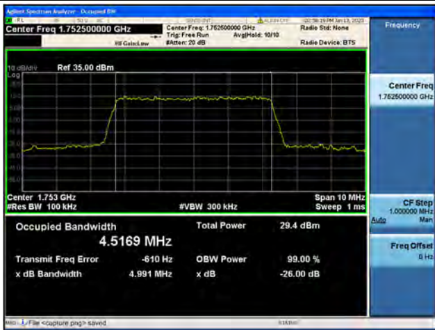
Band4 / 5MHz / 64QAM/ High CH
