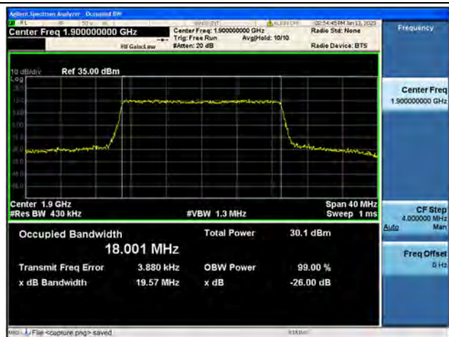
Band2 / 20MHz / 16QAM/ High CH
