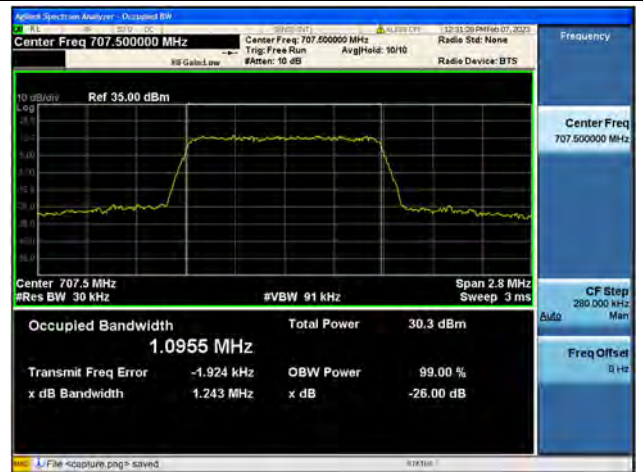
Band12 / 1.4MHz / QPSK/ Mid CH
