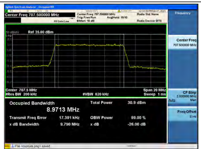
Band12 / 10MHz / 16QAM/ Mid CH
