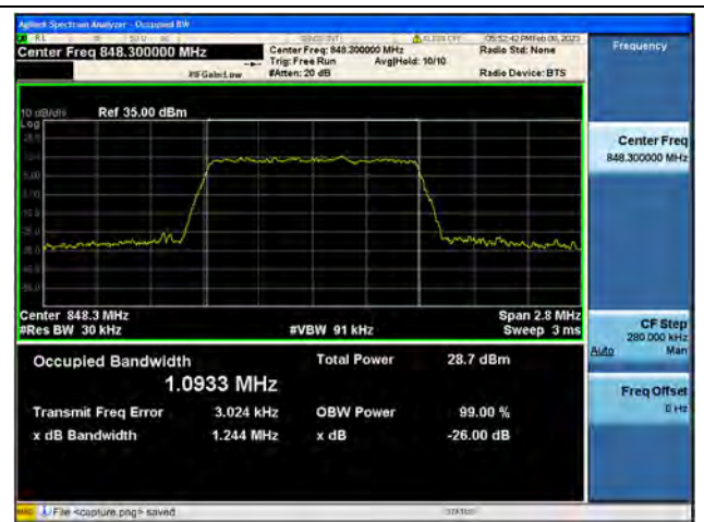
Band5 / 1.4MHz / 16QAM/ High CH
