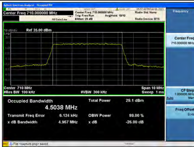
Band17 / 5MHz / 16QAM/ Mid CH
