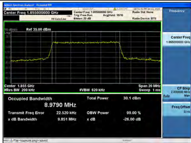
Band2 / 10MHz / 16QAM/ Low CH
