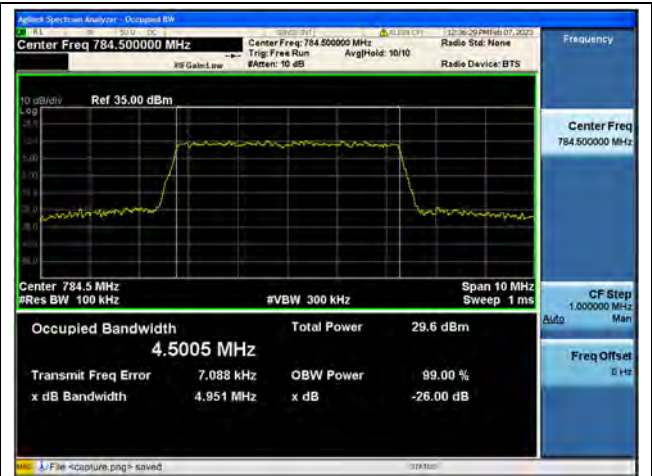
Band13 / 5MHz / 16QAM/ High CH
