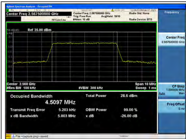
Band7 / 5MHz / QPSK / High CH
