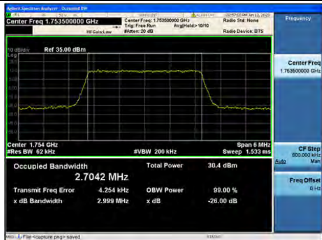
Band4 / 3MHz / 16QAM/ High CH
