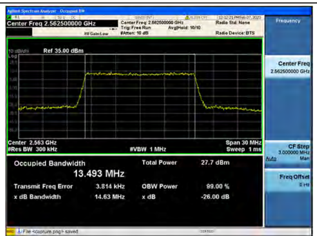
Band7 / 15MHz / 16QAM/ High CH
