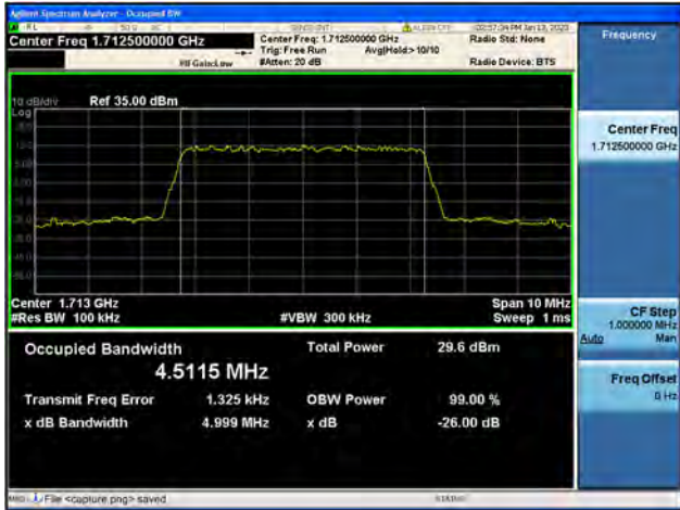
Band4 / 5MHz / 64QAM/ Low CH
