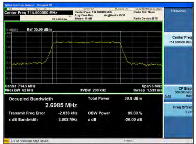
Band12 / 3MHz / QPSK/ High CH
