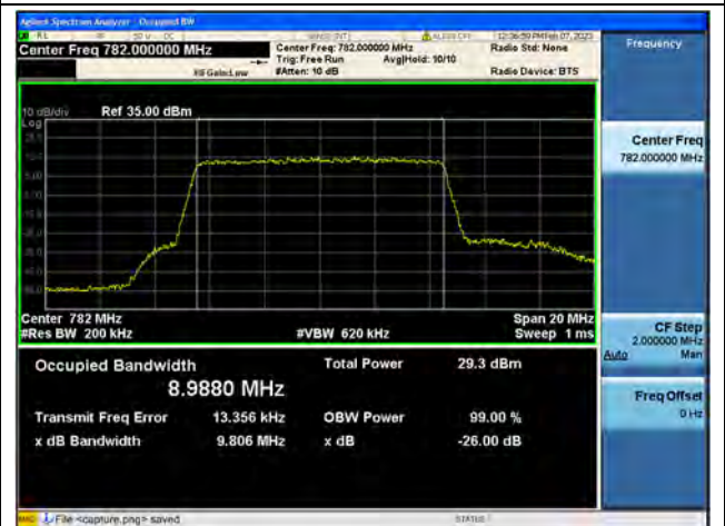
Band13 / 10MHz / 64QAM/ Low CH
