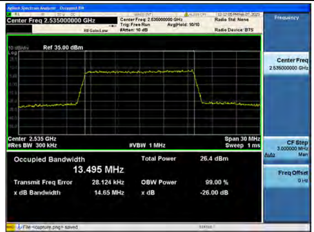
Band7 / 15MHz / 64QAM/ Mid CH
