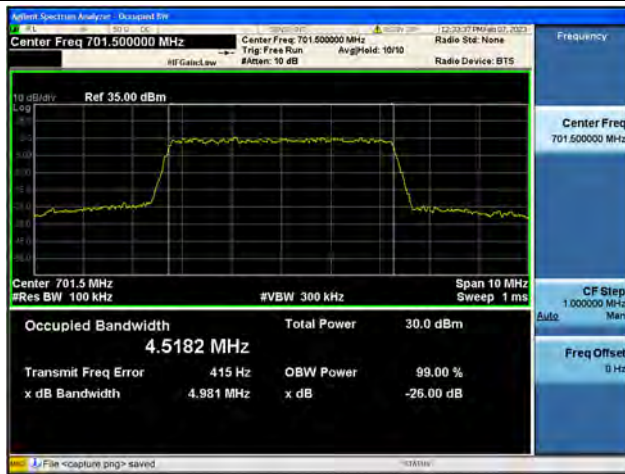
Band12 / 5MHz / 64QAM/ Low CH
