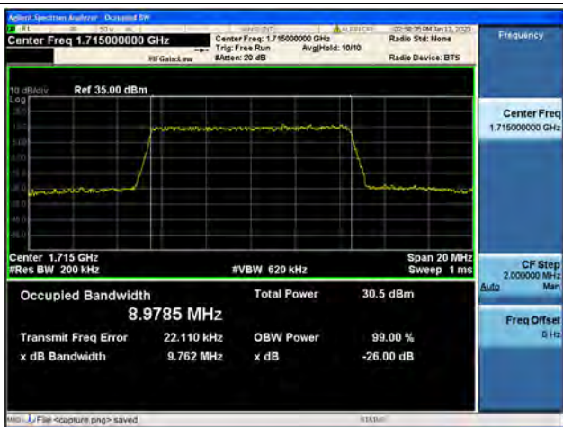
Band4 / 10MHz / 16QAM/ Low CH
