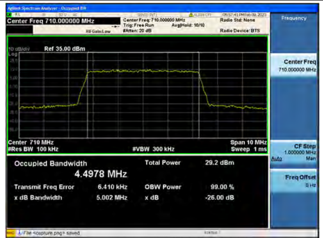
Band17 / 5MHz / QPSK/ Mid CH
