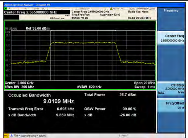
Band7 / 10MHz / 64QAM/ High CH
