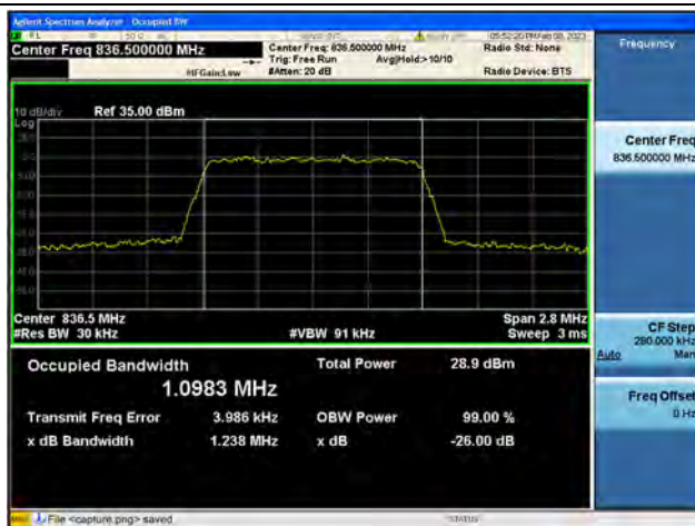
Band5 / 1.4MHz / 16QAM/ Mid CH
