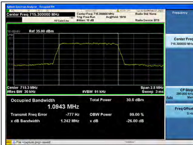
Band12 / 1.4MHz / QPSK/ High CH
