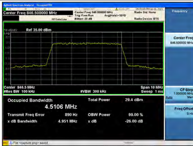
Band5 / 5MHz / 64QAM/ High CH
