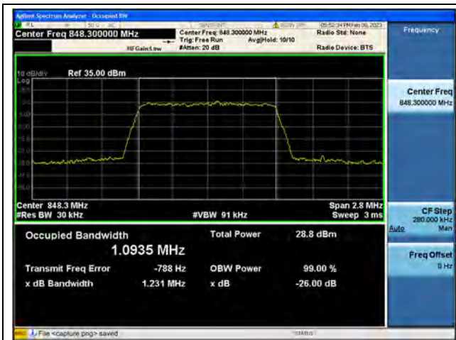
Band5 / 1.4MHz / QPSK/ High CH
