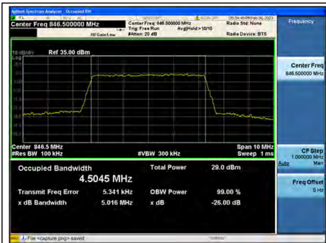
Band5 / 5MHz / QPSK/ High CH
