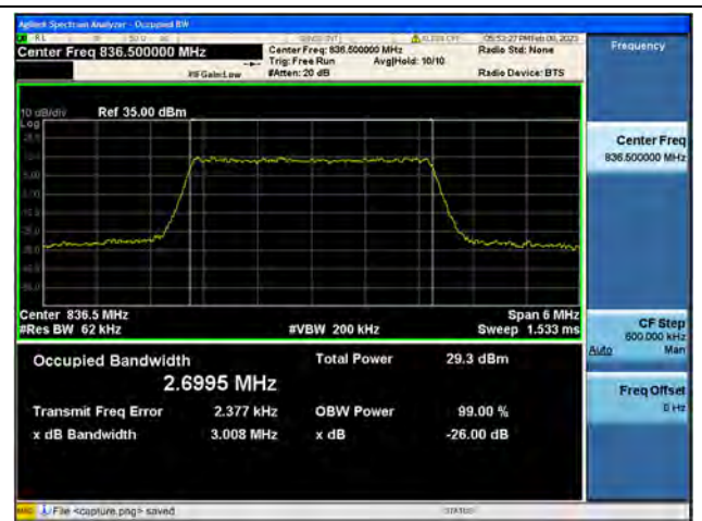
Band5 / 3MHz / 16QAM/ Mid CH
