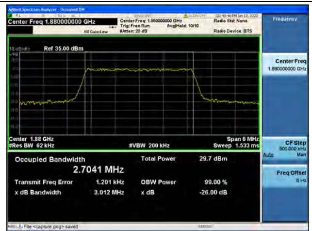
Band2 / 3MHz / 16QAM/ Mid CH
