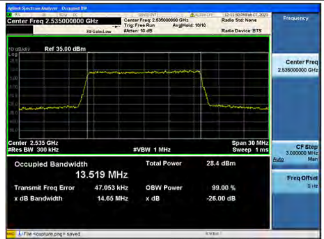
Band7 / 15MHz / QPSK/ Mid CH
