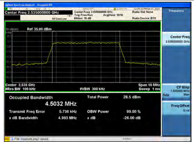
Band7 / 5MHz / QPSK/ Mid CH
