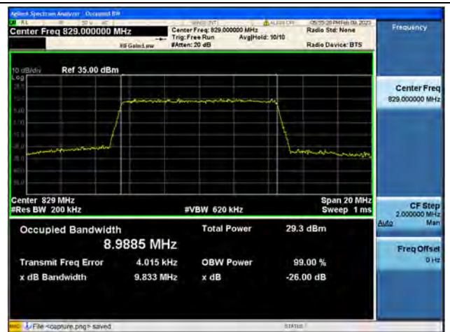
Band5 / 10MHz / 64QAM/ Low CH
