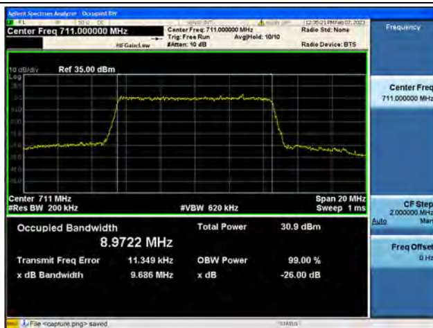
Band12 / 10MHz / 16QAM/ High CH
