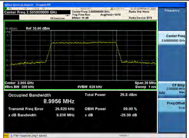
Band7 / 10MHz / 64QAM / Low CH
