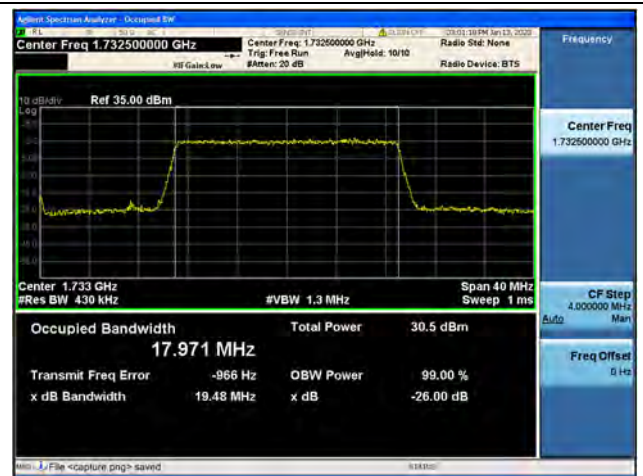
Band4 / 20MHz / 16QAM/ Mid CH
