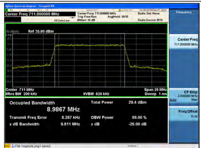
Band12 / 10MHz / 64QAM/ High CH
