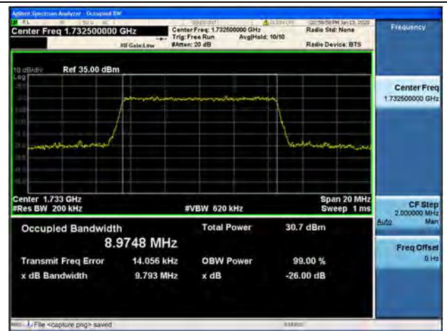
Band4 / 10MHz / 16QAM/ Mid CH
