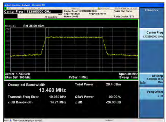
Band4 / 15MHz / 64QAM/ Mid CH
