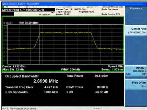
Band4 / 3MHz / 16QAM/ Low CH
