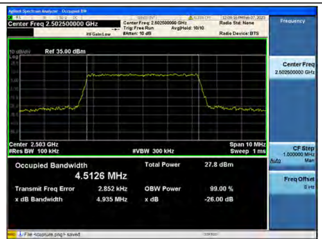
Band7 / 5MHz / 16QAM/ Low CH
