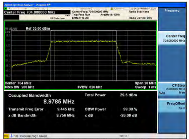
Band12 / 10MHz / QPSK/ Low CH
