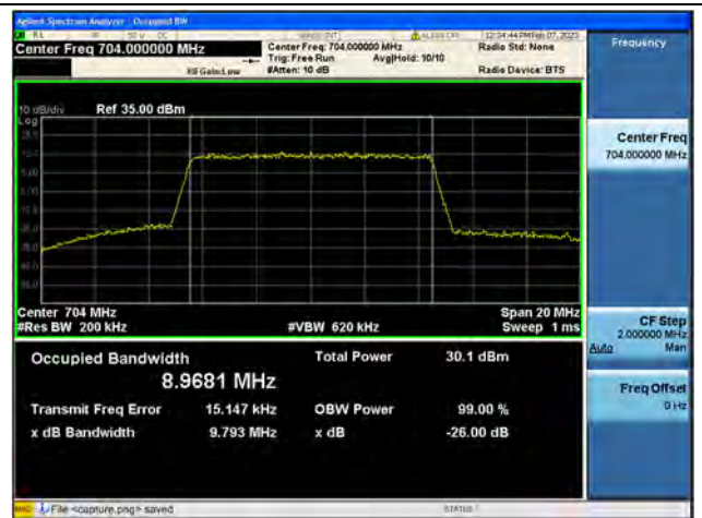
Band12 / 10MHz / 64QAM/ Low CH
