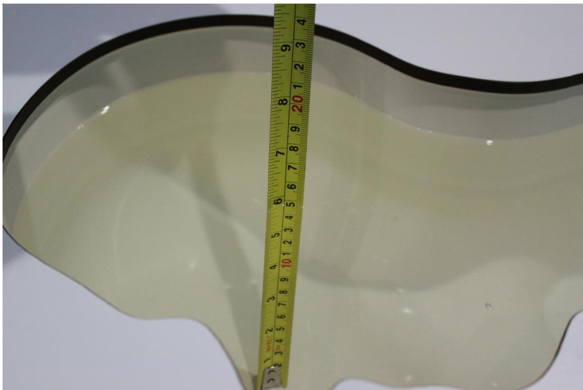
Picture 8-6 Liquid depth in the Head Phantom (5GHz)
