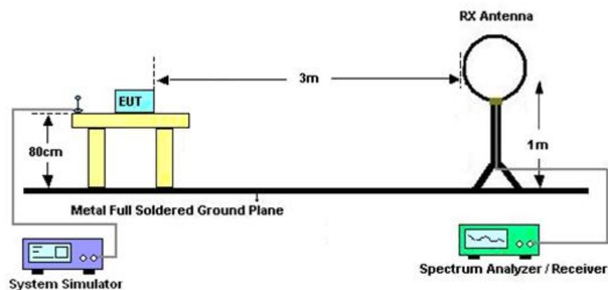
For radiated emissions from 30MHz to 1GHz
