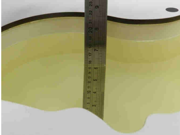
Fig 10.1 Photo of Liquid Height for Head SAR
