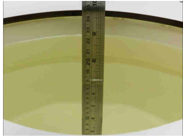
Fig 10.2 Photo of Liquid Height for Body SAR
