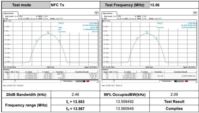
**Remark:** Because the measured signal is CW/CW-like adjusting the RBW per C63.10 would not be practical since measured bandwidth will always follow the RBW and the result will be approximately twice the RBW
