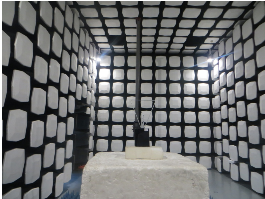
Pic.1 Radiated spurious emission(below 3GHz)
