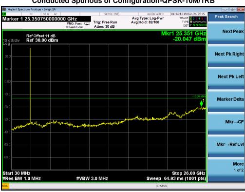
Conducted Spurious of Configuration-QPSK-10M/1RB
