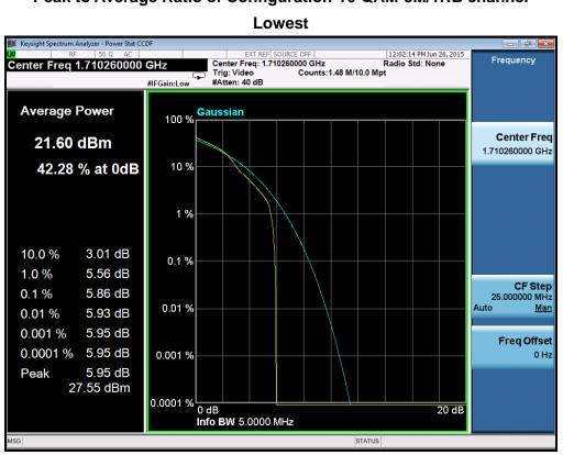
Peak to Average Ratio of Configuration-16-QAM-3M/1RB channel
