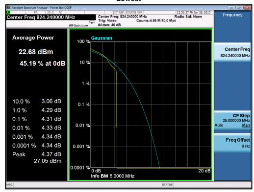
Peak to Average Radio of Configuration-16-QAM-1.4M/1RB channel Middle
