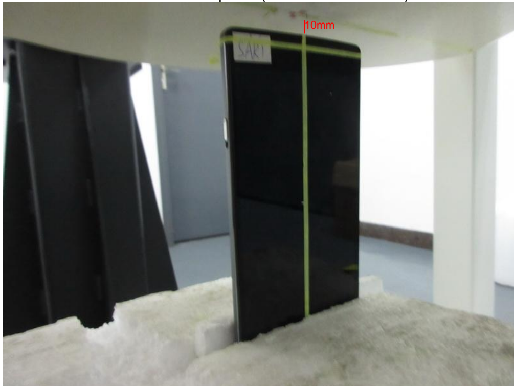
Test Position Top Side(Test distance=10mm)
