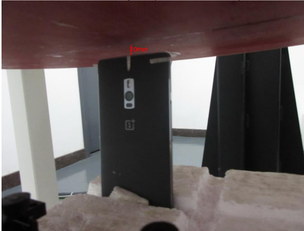
Test Position Top Side(Test distance=10mm)
