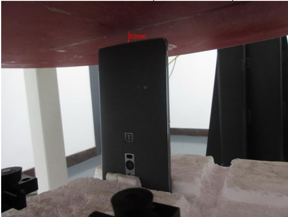
Test Position Bottom Side(Test distance=10mm)
