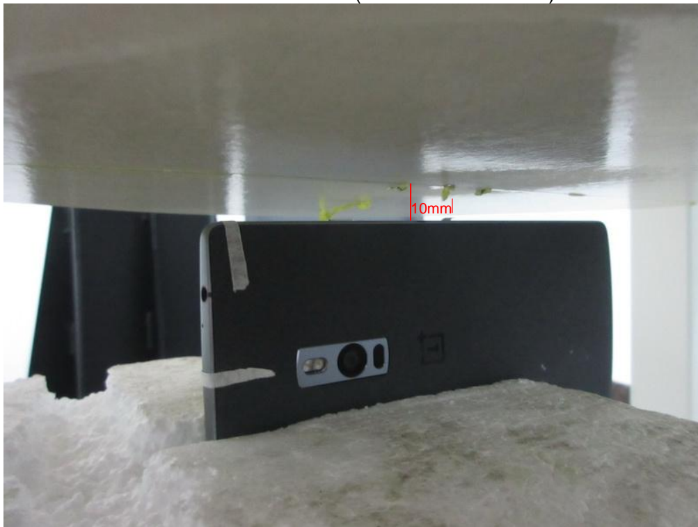
Test Position Left Side(Test distance=10mm)
