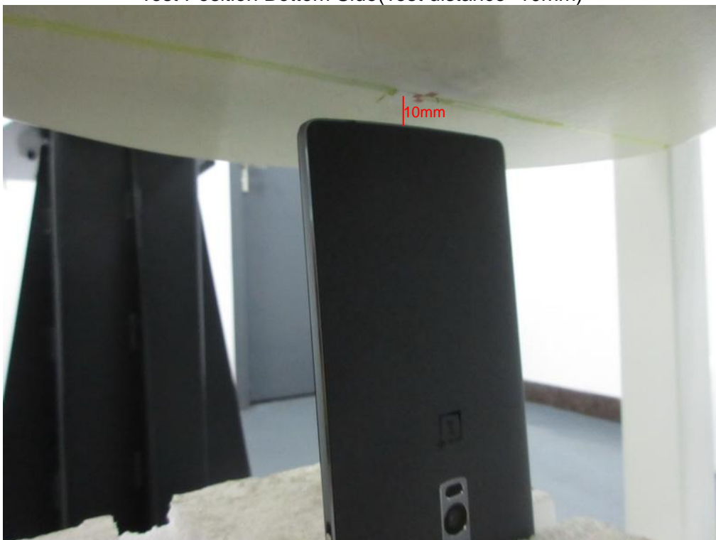
Test Position Bottom Side(Test distance=10mm)
