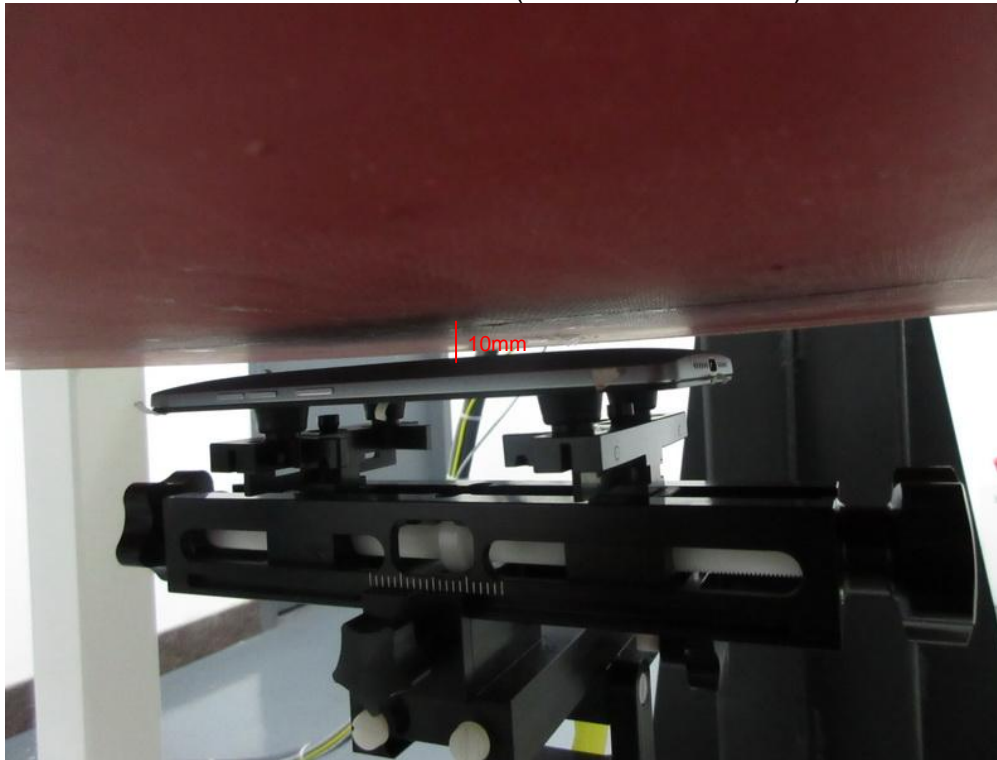
Test Position Rear Face(Test distance=10mm)
