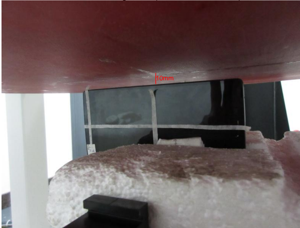
Test Position Right Side(Test distance=10mm)
