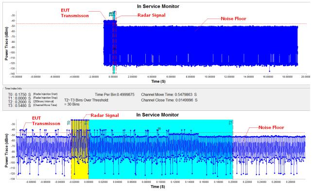
**Note:** T0 denotes the start of Channel Move Time upon the end of the last Radar burst.
