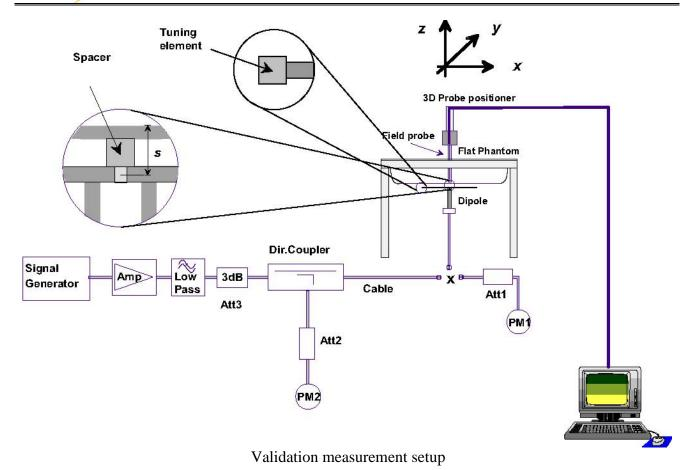
For the waveguide measurement, the distance s=0mm (waveguide is in contact with the phantom)
