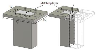
Figure 1: Validation Waveguide Dimensions
