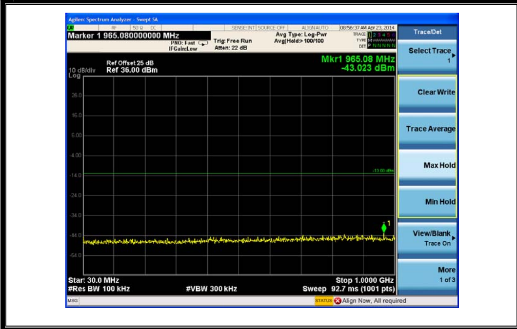
(Plot P1: HSPA+1700MHz Channel = 1312, 30MHz to 1GHz)
