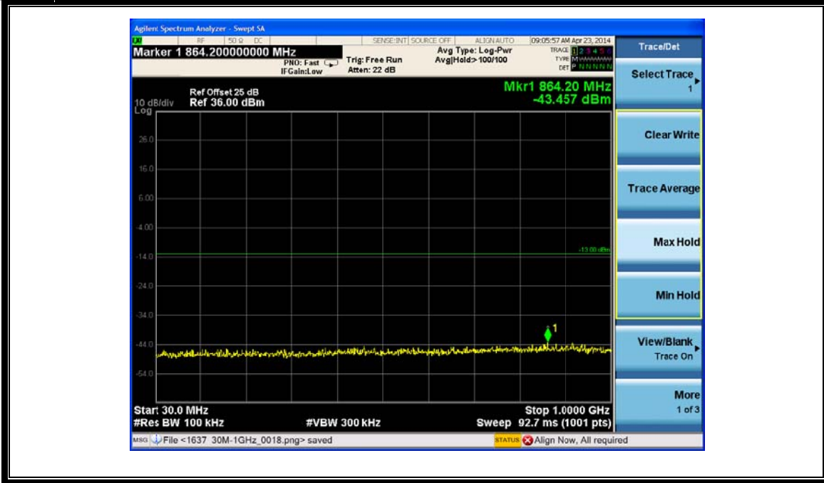
(Plot N3: HSDPA1700MHz Channel = 1513, 30MHz to 1GHz)
