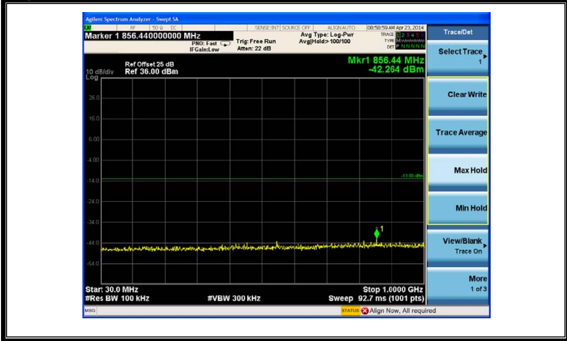
(Plot P3: HSPA+1700MHz Channel = 1513, 30MHz to 1GHz)
