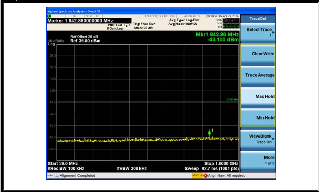
(Plot N1: HSDPA1700MHz Channel = 1312, 30MHz to 1GHz)
