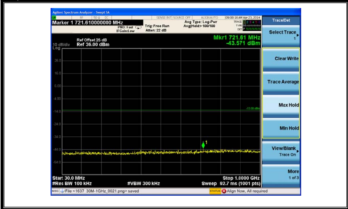
(Plot M1: WCDMA1700MHz Channel = 1312, 30MHz to 1GHz)
