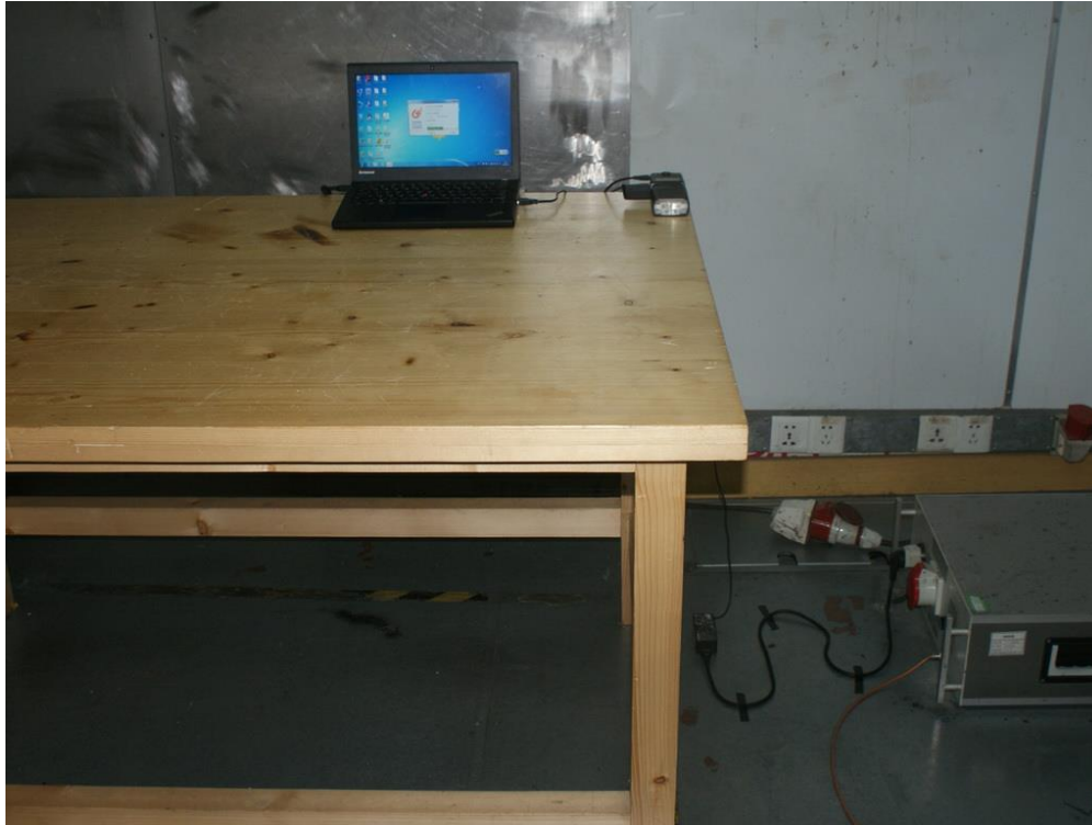
Photograph 5: Set-up for Conducted Emissions
