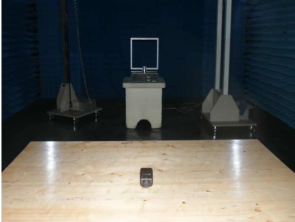
Photograph 2: Set-up for Spurious Emissions (30MHz-1GHz)
