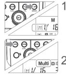
Press the <SLAVE> Button to choose the group from M/A/B/C. Then, press the < MODE > Button so that the master unit can work in OFF / TTL / M flash mode Choose one of them as the flash mode of master unit
